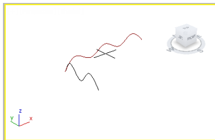
Figure 15-53 The curves to create 1-rail surface
