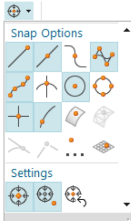
Figure 2-49 The Snap Point flyout used for snap settings
