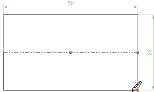
Figure 2-24 Rectangle being drawn by using the centerpoint method
