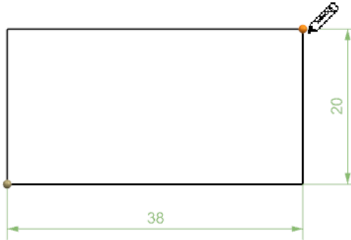
Figure 2-23 Rectangle being drawn by using the By 2 Points method
