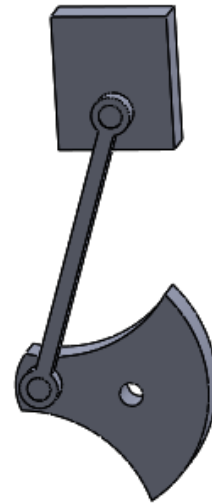
Figure 2-37 Reciprocating mechanism after hiding the sketches
