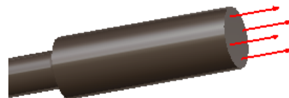
Figure 19-130 The User-defined Restraint applied to the selected face
